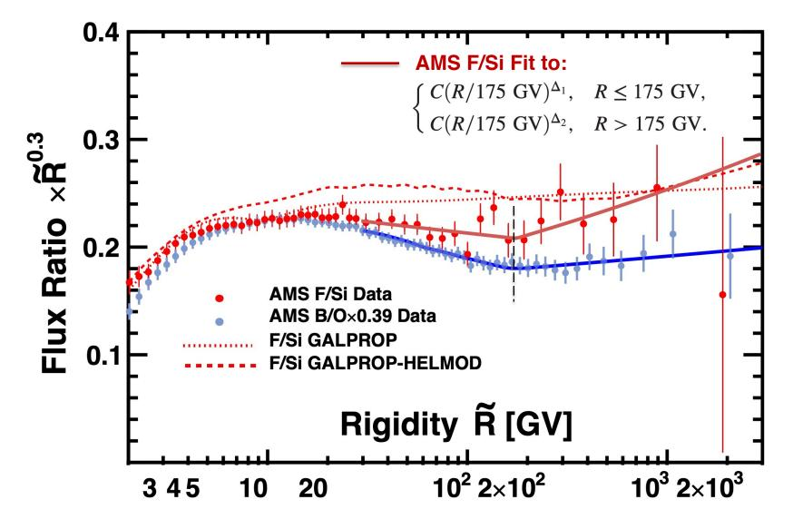
Above 175 GV, the F/Si ratio exhibits a hardening  $(\Delta_2^{F/Si} - \Delta_1^{F/Si})$  of 0.15  $\pm$  0.07 compatible with the AMS result on the hardening of the Li/O, Be/O, and B/O flux ratios.
