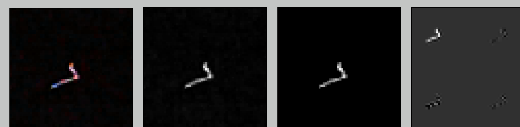
Fig. 3: Example of the worm-type image. Left to right: original image (color), grayscale accumulation, adaptive thresholding and Daubechies wavelet transformation.
