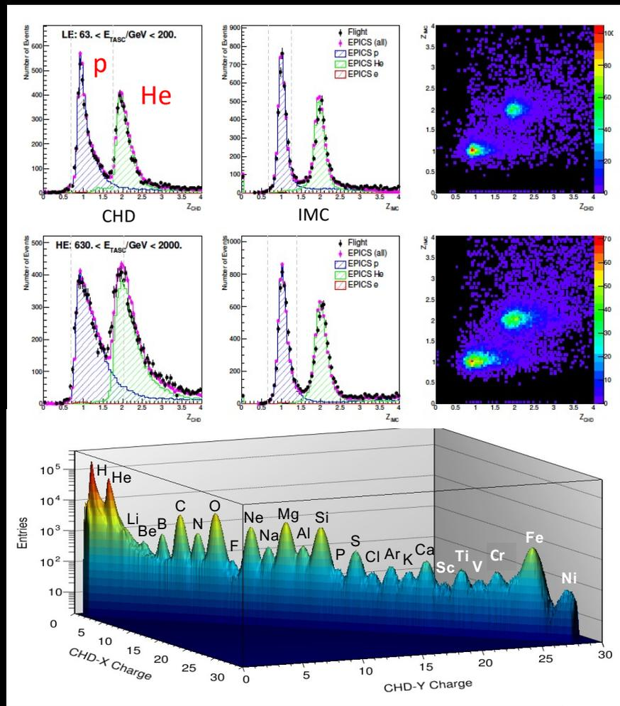
Deviation from  $Z^2$  response is corrected both in CHD and IMC using a core + halo ionization model (Voltz)
