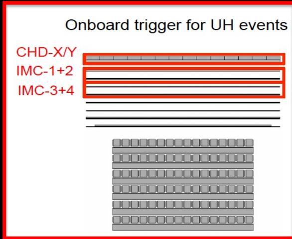
A special UH CR trigger uses the CHD and the first 4 layers of the IMC to achieve an expanded  $\times 4$  geometric factor
