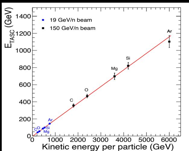
← Beam calibrations at CERN-SPS with ion fragments at 13, 19, 150 GeV/n
