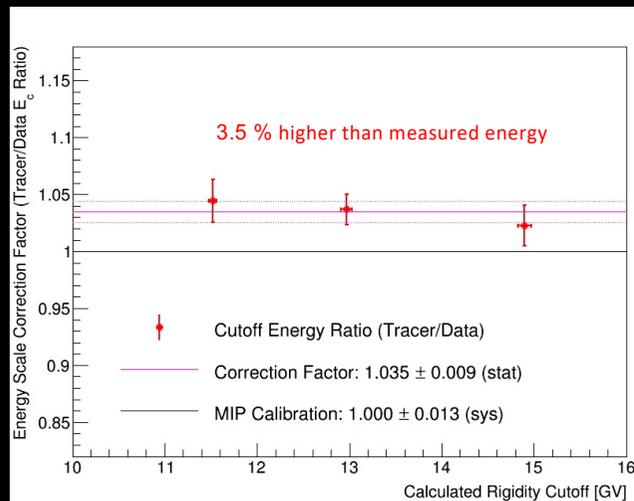
← Absolute energy scale calibration for electrons using rigidity cutoff
