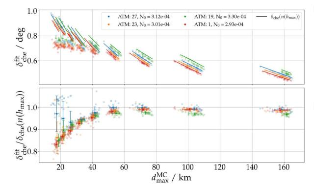
position of Gauss corresponds to Cherenkov radius calculated from refractive index at Xmax!
