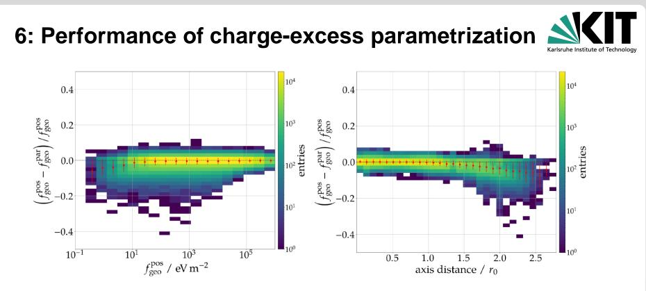
agreement of charge-excess parameterization with direct calculation agrees on average within 2%
