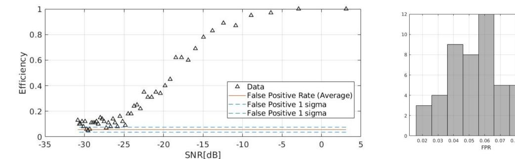
We can assume that above -15 dB, the efficiency is almost 90%, with a very low and constant **FPR** ~ 6% per 2082 samples, or ~15 kHz (for a 500 MHz sampling rate [2] of the GRAND experiment).
