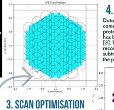
The time taken to calibrate the camera depends on the vertical and horizontal movement of screen. The screen positions are shown using red outlines, the path of the screen as dotted line. The limit of the motors are signified by the black lines. The velocity and acceleration of motors result in 55 scan positions with scanning time ranging from 17 to 28 minutes.
