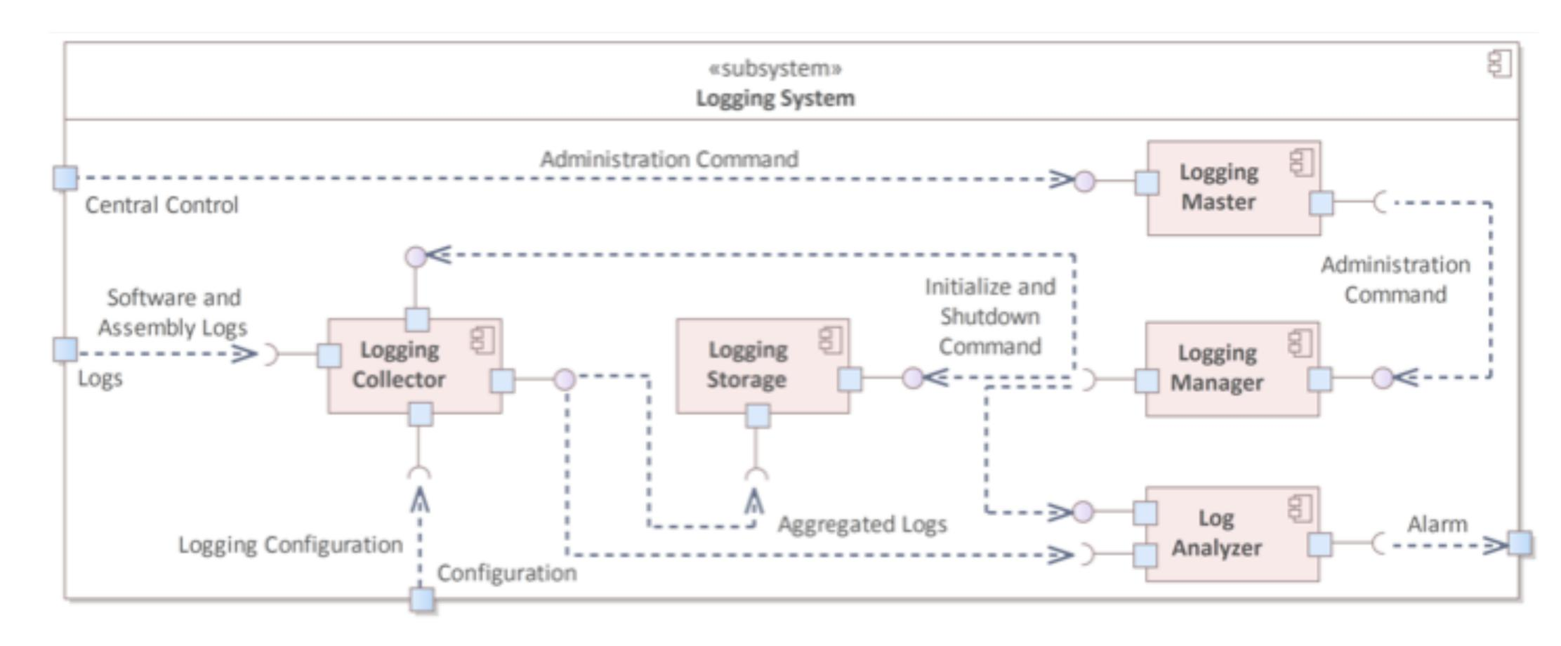
Fig. 1: Logical view of LOUD. Log sources are Alma Common Software (ACS) components, OPC UA servers and low-level software.
