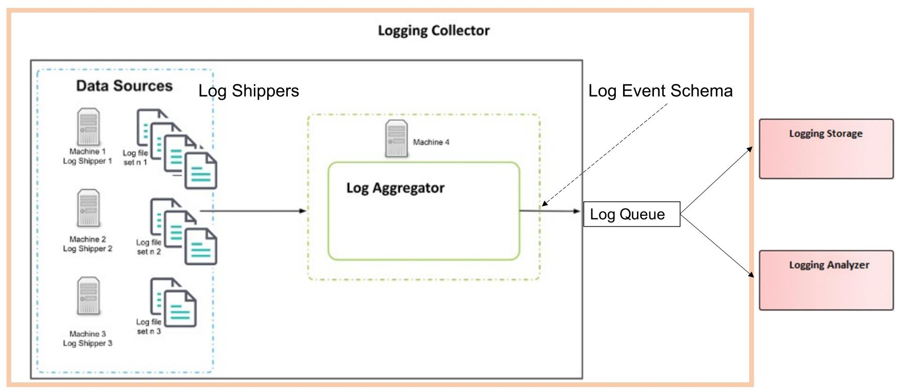
Fig. 2: Architecture of the Logging Collector.
