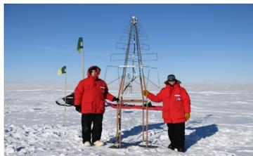
\*Antennas and Scintillators are elevated to avoid snow coverage
