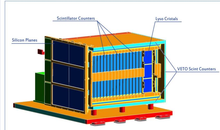
The High-Energy Particle Detector (HEPD-01), developed by the Italian Collaboration, detects electrons, protons and light nuclei. The main objective is to measure the increase of the electron and proton fluxes due to short-time perturbations of the radiation belts caused by solar, terrestrial and anthropic phenomena. The energy range explored is 3 - 100 MeV for electrons and 30 - 200 MeV for protons.
