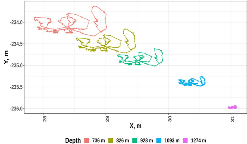
OM drift can reach tens of meters, depends on season and elevation.
