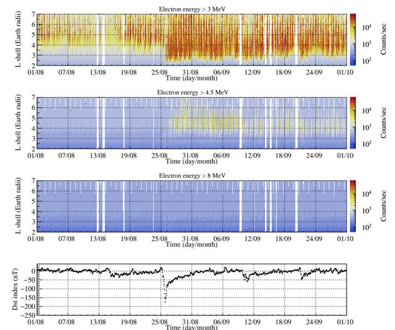
Fig.3: Top three panels: Trigger rates for three different HEPD-01 configurations over the period August-September 2018. Bottom panel: Time evolution of the Disturbance storm-time index.
