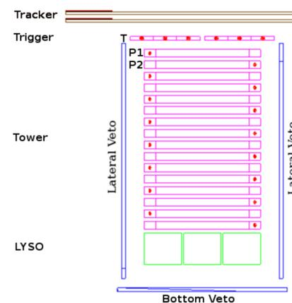
Fig.1: Schematic of the HEPD-01 detector.
