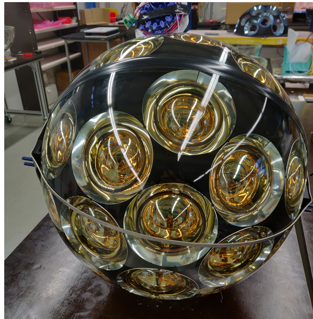
Optical modules with 31 PMTs
