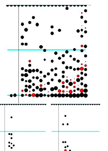
We record the time of each interaction to an accuracy of two microseconds and are able to form "images" of complex interactions. Here we show an actual air shower core (top) and two simulated 100 GeV neutrons.
