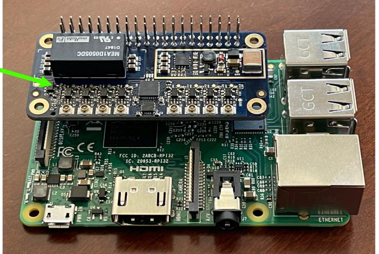
An 8-channel FPGA board is developed for the raspberry PI based readout. This PCB also supplies the bias voltage for the SiPMs. More sensors can be added, e.g. GPS sensor, etc
