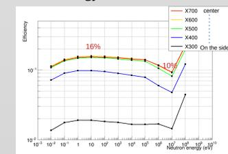
Fig. 8. Simulated registration efficiency of monoenergetic neutrons for neutron counters from the central one to the most to the side.
