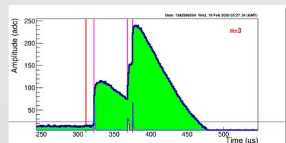
Fig. 1 Example of multiple neutron signal registered in single <sup>3</sup>He counter.
