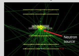
Fig. 7. Geant4 schematic view presenting 100 neutron tracks for neutron transport and detection simulations. 10 MeV neutrons are emitted isotropically from the same position in lead.
