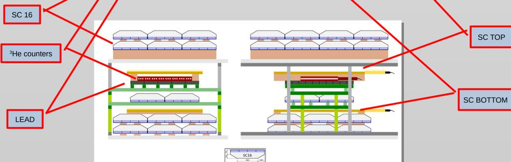
Fig. 2. Our detector set-up: Front and side views. System is operating since October 2019. EMMA hodoscopic detectors (in grey) form 5 layers. Dark gray layer in the center is made of 5cm lead bricks. Above it there are polyethylene blocks with 14 helium neutron counters (in white holes). Yellow layers are 2 scintillation detectors 1m<sup>2</sup> each.
