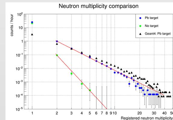
Fig. 6. Neutron multiplicity spectra collected during run with lead target (Blue dots) and without target (green dots). Red lines - power function fit (tab. 1).
