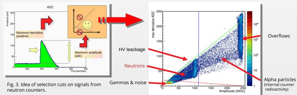
Fig. 3. Idea of selection cuts on signals from neutron counters.
