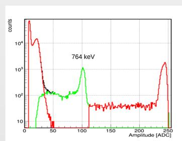
Fig. 5. Amplitude spectra from single <sup>3</sup>He neutron counter. Green line represent neutron signals, black - all signals, red - rejected by cuts.
