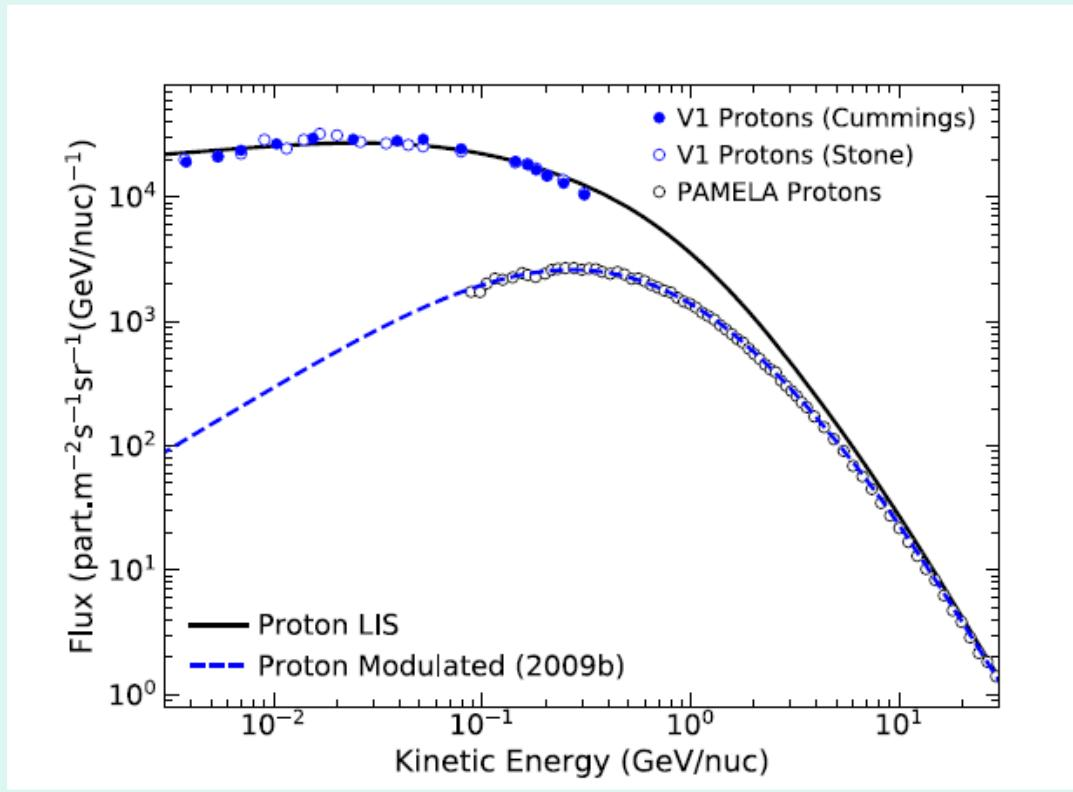
$$J_p(E) = 2620.0 \frac{1}{\beta^2} \left( \frac{E}{E_0} \right)^{1.1} \left( \frac{(E/E_0)^{0.98} + 0.7^{0.98}}{1 + 0.7^{0.98}} \right)^{-4.0} + 30.0 \left( \frac{E}{E_0} \right)^2 \left( \frac{E/E_0 + 8.0}{9.0} \right)^{-12.0},$$
