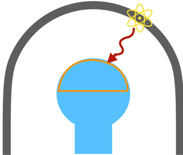
**PMT dark rate impacted by glass refractive index boundary**
