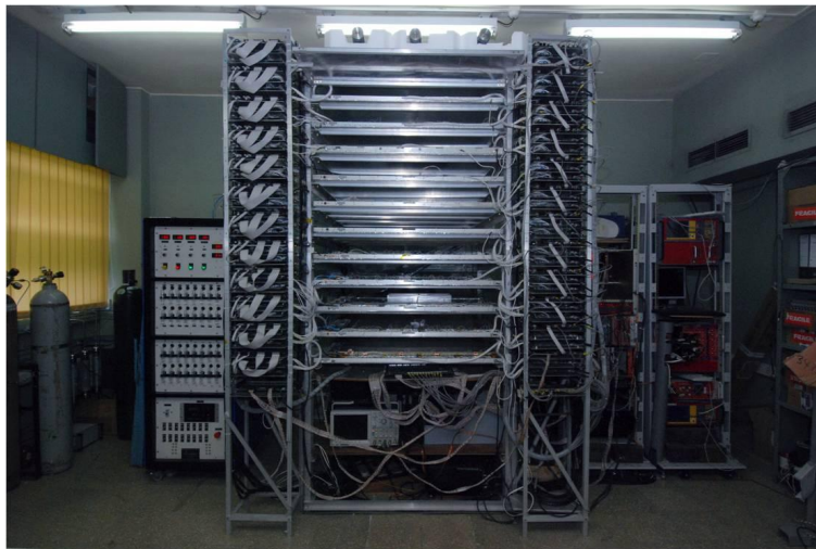
Fig 3. 1m x 1m RPC stack at TIFR
