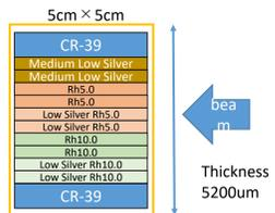
Fig3. Detector consists of emulsion and CR-39.
