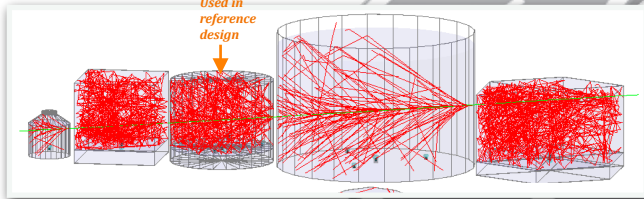
Figure 1: Different available GEANT4 tank types. Shown are a fraction of the Cherenkov photon tracks generated by a muon traveling from left to right
