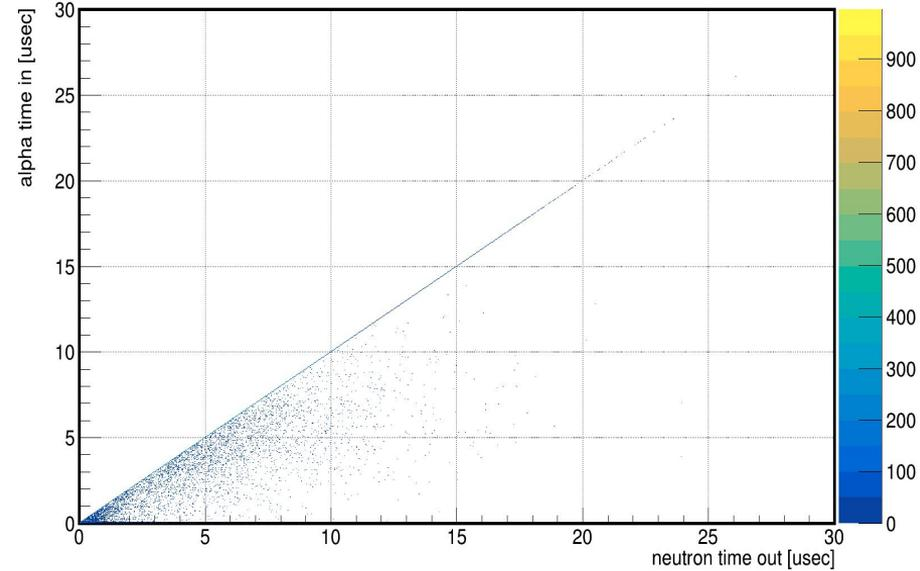
**The correlation between time moment, when the last alpha particle are born in an event and the time moment when the last neutron leave the detector or it was absorbed by It**
