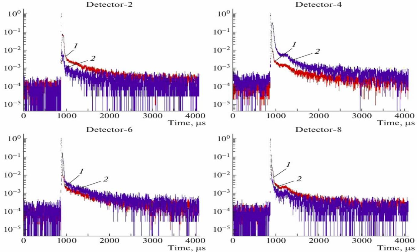
The time dependence of the neutron signals in the downstream BS detectors: (1) after the prototype shift, (2) before the prototype shift.
