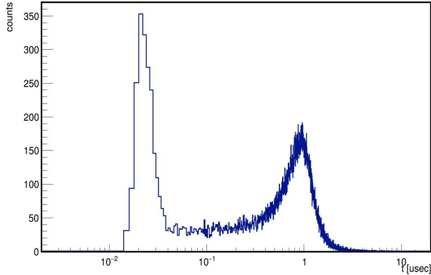
**The average lifetimes of evaporated neutrons inside of the detector for the different energies of incoming protons**
