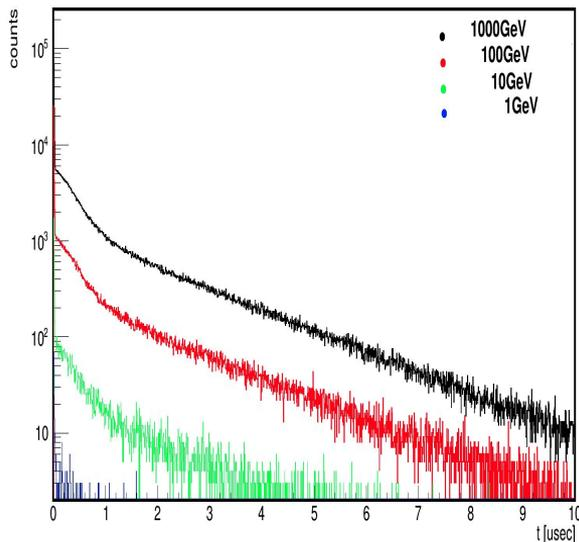
The lifetime distributions of evaporated neutrons inside of the detector for the different energies of incoming protons.
