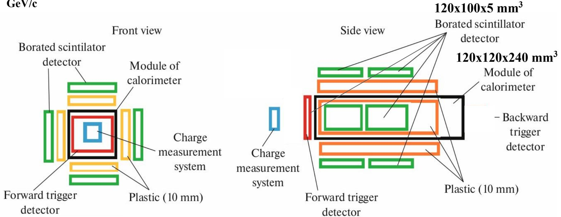
OLVE-HERO prototype scheme on the beam test experiment at SPS CERN.
