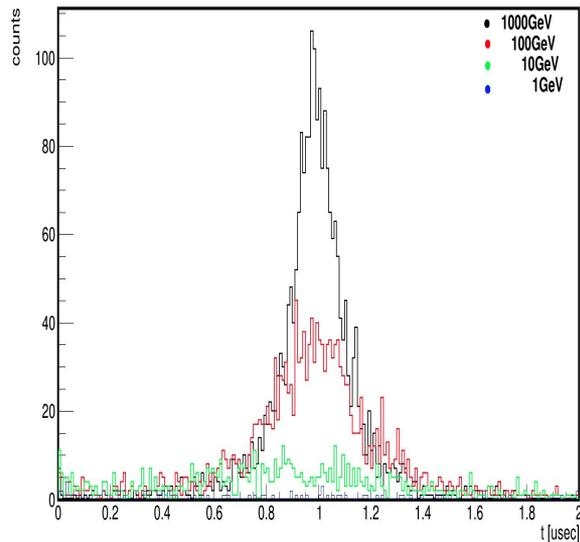
The average lifetimes of evaporated neutrons inside of the detector for the different energies of incoming protons
