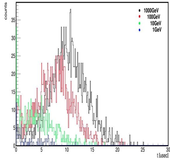
The time distributions of the last evaporated neutrons for the different energies of incoming protons
