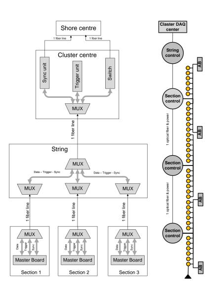
For DAQ implementation the CWDM technology (Coarse Wavelength Division Multiplexing) was applied. This approach makes it possible to transmit all information (the data stream, trigger, and sync) over a single optical fiber, which allows to limit each segment of the underwater network to one fiber-optic line.
