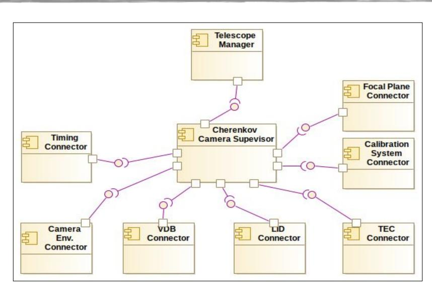
Figure 2: Cherenkov Camera Supervisor UML Component Diagram
