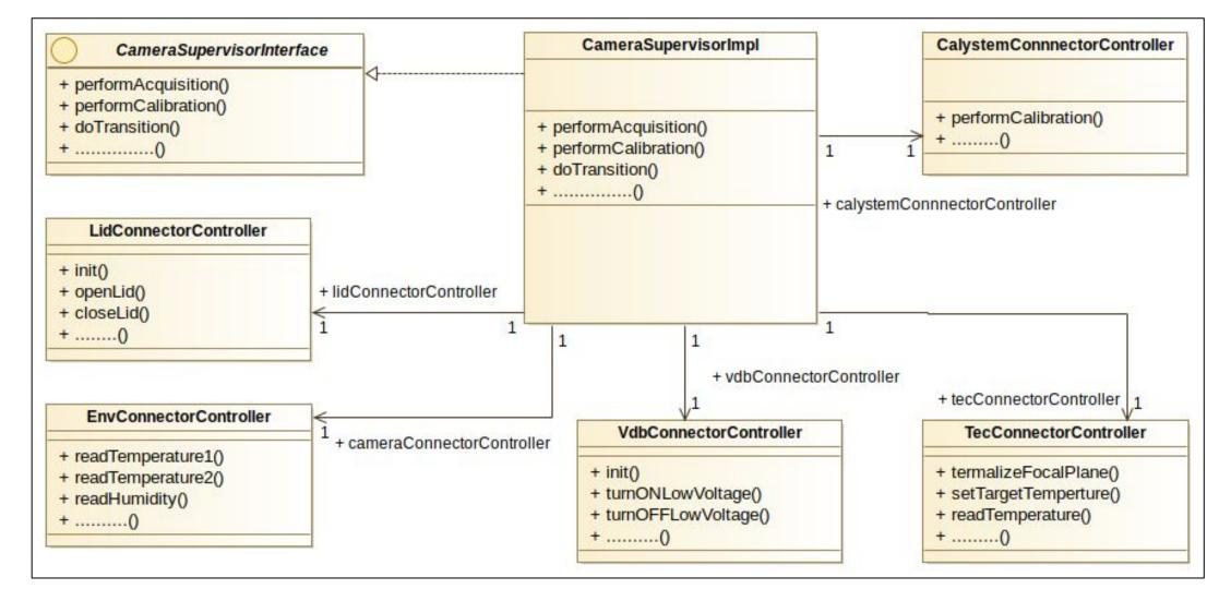
Figure 3: Cherenkov Camera Supervisor UML Class Diagram
