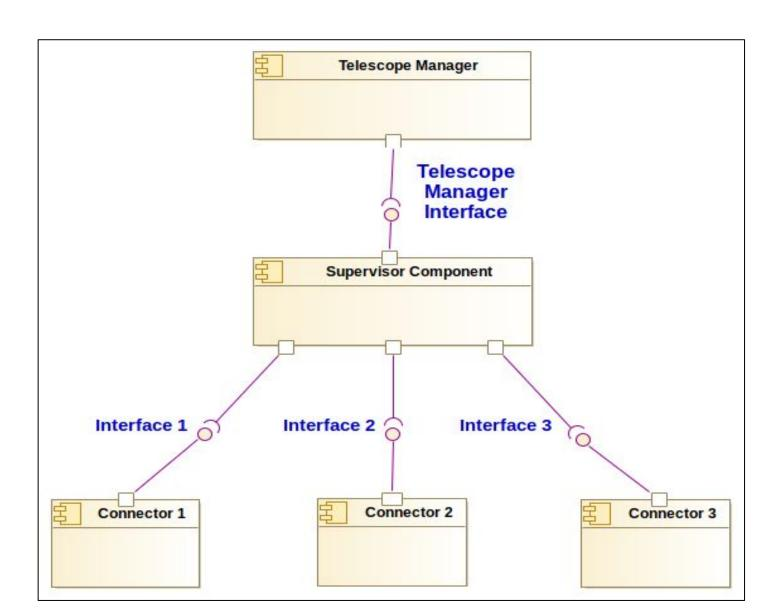
Figure 1: UML Component Diagram of Telescope Control System
