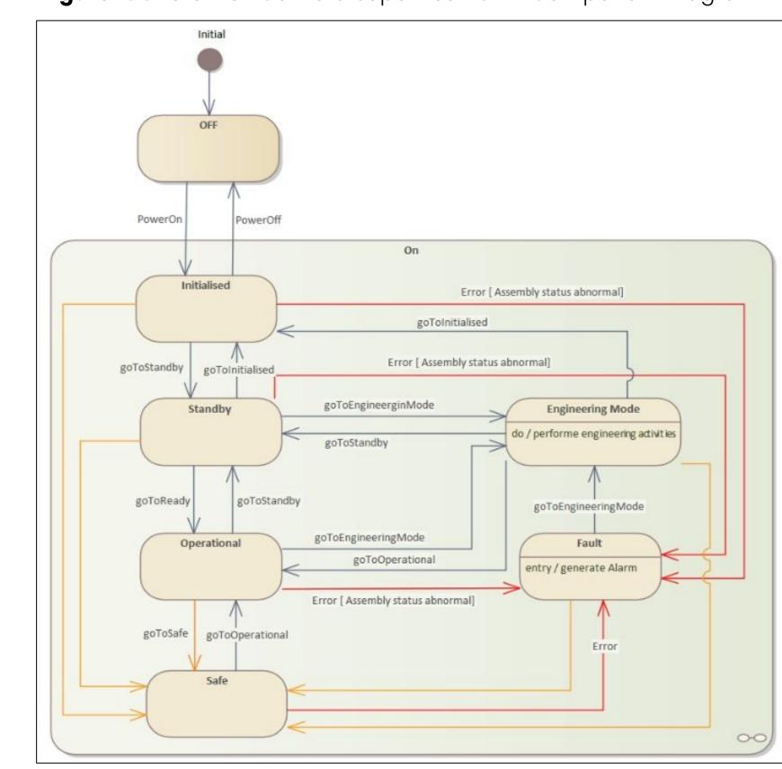
Figure 4: Cherenkov Camera Supervisor State Machine
