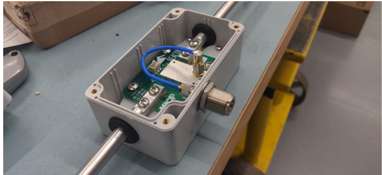
A short dipole active feed enclosure (open for display). This antenna was installed during the June 2021 deployment.
