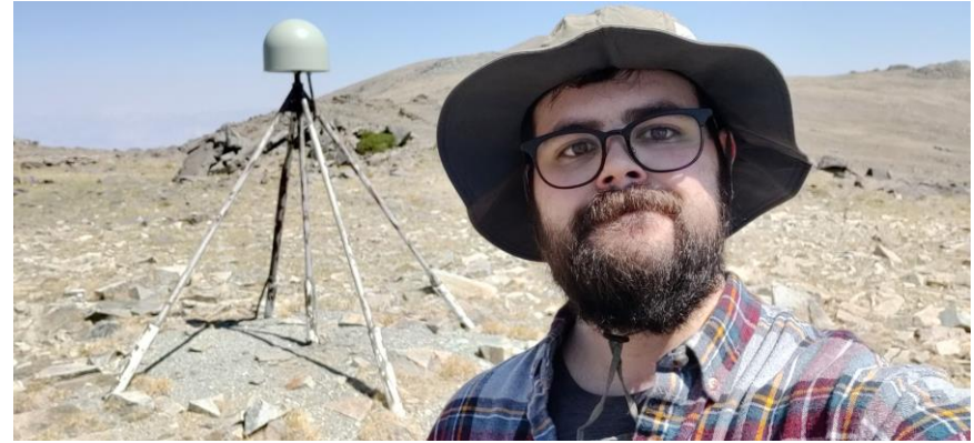
NTRIP Corrective GPS data provided by UNAVCO GPS Station P652, conveniently installed ~ 30m from our closest BEACON prototype mast
