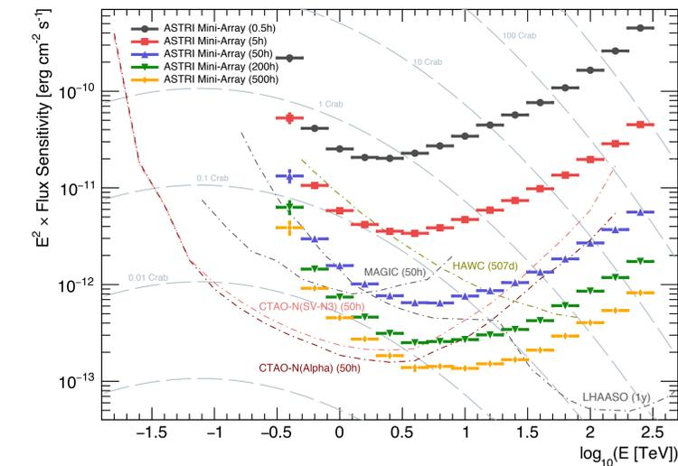
**Figure 2:** On-axis point-like source differential sensitivity of the ASTRI MA (at a zenith angle of 20°) for five exposure times: 0.5 (dark gray), 5 (red), 50 (blue), 200 (green), and 500 (orange) hours. The differential sensitivities of other instruments – MAGIC (50h), HAWC (507d), LHAASO (1y), and CTAO Northern Array (50h, for two configurations) – are shown for comparison.
