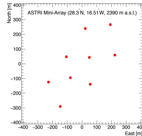
**Figure 1:** Layout of the ASTRI MA telescopes at the Teide Observatory site.
