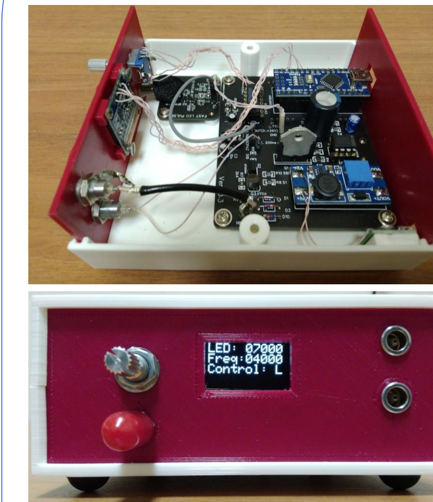
Figure 3: Stand-alone desktop module of fast light pulses source for calibration of the 0.5-t prototype of the Large Baksan Neutrino Telescope project: front view and without cover.
