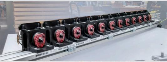
Figure 2: PMTs on a slide-in bar
