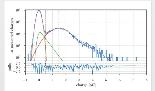
Figure 6: Example of a recorded SPE spectrum
