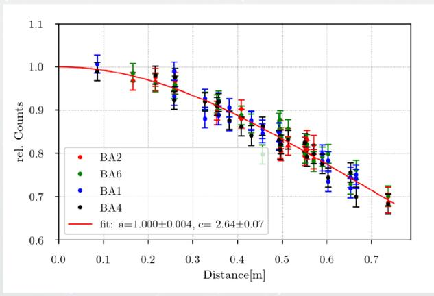
Figure 5: Relative light yield as a function of distance to the PMT rack center. From [9].
