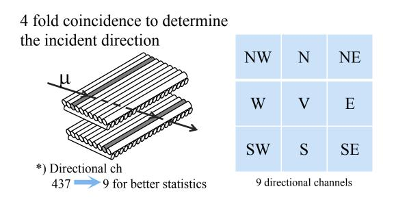
A 3NM64 was installed in each of the two containers. A MD was constructed beneath the 3NM64, only in one container. (left top & left bottom) To analyze Syowa MD data with better statistics, 437 directional channels are combined into 9 channels (above).
