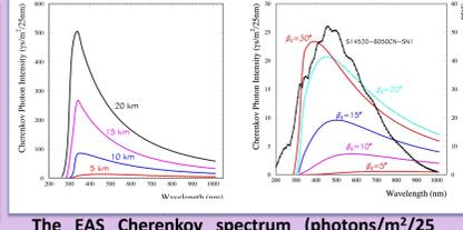
The EAS Cherenkov spectrum (photons/m<sup>2</sup>/25 nm) at 525 km altitude for a 100 PeV upward EAS for  $\beta_{tr} = 10^\circ$ . Left: versus EAS starting altitude Right: versus  $\beta_{tr}$ . The measured PDE curve of a representative SiPM is overlaid. Ref: JCAP V2021, 106, id007.
