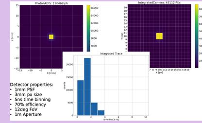
Example of the modeling of a pixelated optical Cherenkov detector. *Implementation in progress*.
