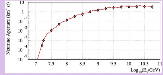
The results of a *vSpaceSim* calculation of  $\nu_\tau$  aperture for the diffuse  $\nu_\tau$  flux for a POEMMA-like detector viewing the surface of the Earth  $7^\circ$  below the limb and  $360^\circ$  in azimuth. The points are from *vSpaceSim* while the red curve is from that used in PhysRevD.100.063010
