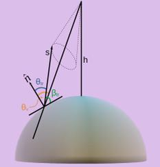
The geometry for observing a  $\tau$ -lepton induced EAS from a detector at altitude  $h$ . See NU ID#482.
