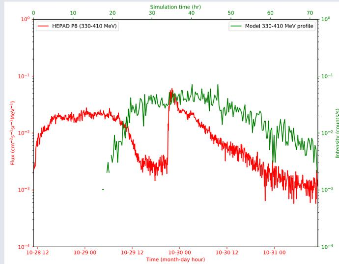
1AU modelled intensity profile at Earth's location
