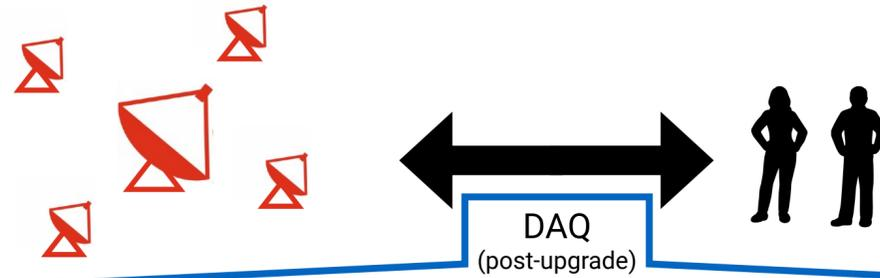
The Data Acquisition System (DAQ) oversees the array operations: telescope movement, data taking and conversion, data storage, etc. It comprises both the hardware and the software.
