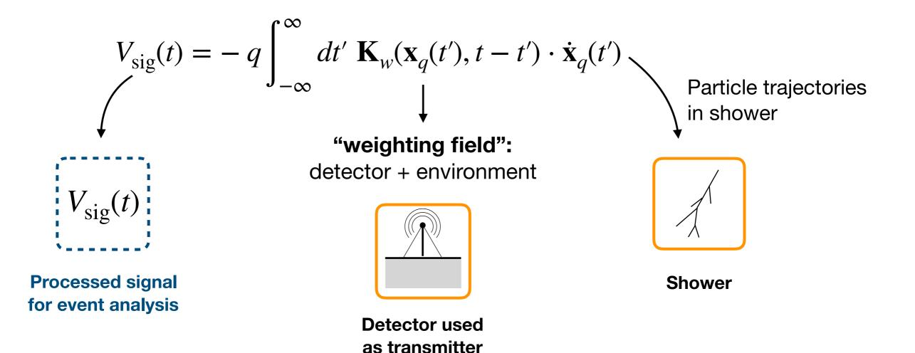
Weighting field precomputed and stored; simulator only performs convolution
