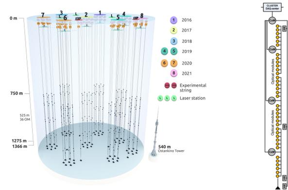
The main component of the OM is a photomultiplier tube with hemispherical photocathode enclosed in pressure-resistant glass sphere with diameter 42 cm. In OM, there is also a controller, a two channel amplifier, two LEDs for time and charge calibrations, and a high-voltage supply.
