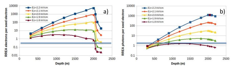
Avalanche started at 5400 m a.s.l. (0 depth), that is 2200 m above the Aragats station. The number of avalanche particles is calculated each 300 m. After exiting from the electric field propagation of avalanche particles is followed additionally 200 m before reaching the station. By blue line, we show the electron and gamma ray number per seed electron for the TGE that occurred on 14 June 2020.
