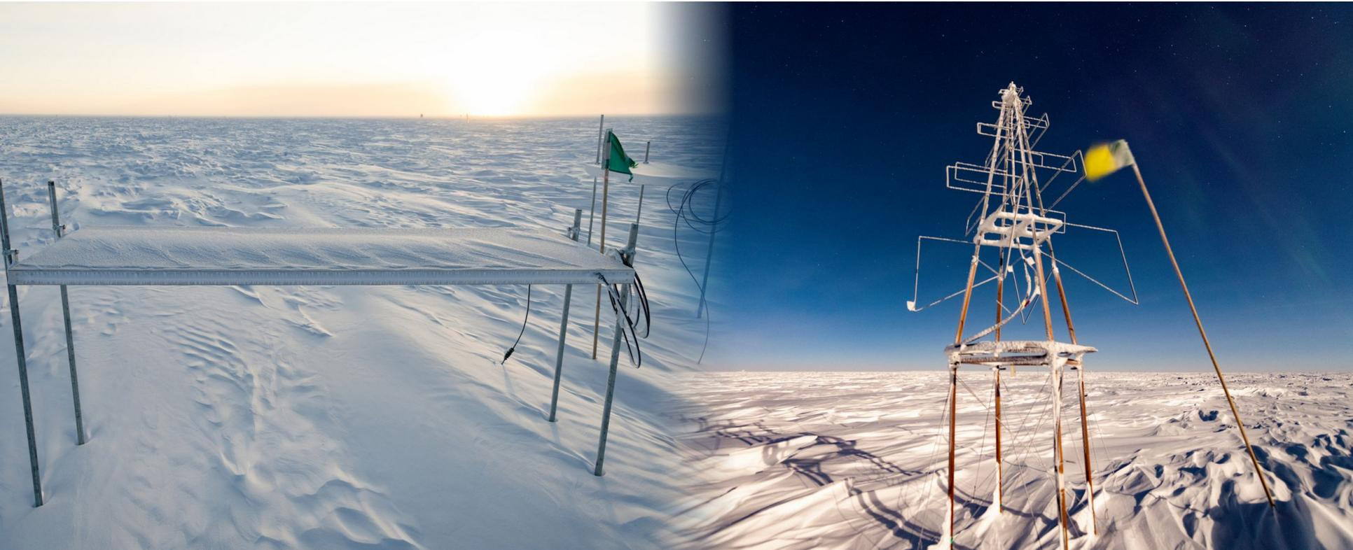
Hybrid station with 8 scintillators and 3 antennas above each in-ice string.
