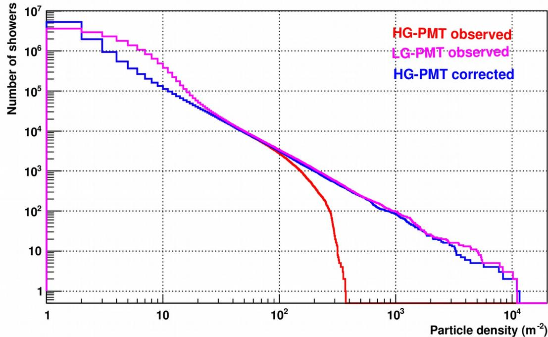
Non-linearity correction enhances particle density measurements of single PMT detectors from 100-200 to over  $5000 \text{ m}^{-2}$
