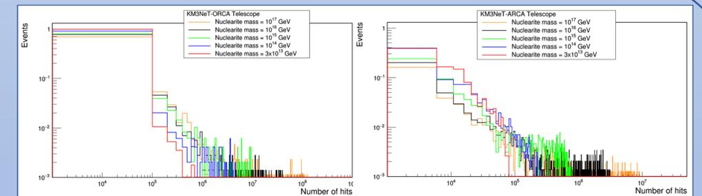
Fig. 4 – Distribution of the number of hits: The distributions show that the number of hits observed depend on the photomultiplier density of the detectors and also it increases with the nuclearite mass.
