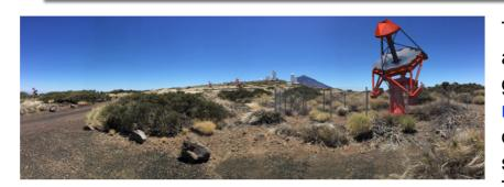
The **ASTRI Mini-Array** (ASTRI-MA) is an INAF project of an array of nine innovative IACTs to study sources emitting gamma-rays in the TeV spectral band [see Antonelli's talk n.832]. Each telescope is characterized by a dual-mirror optical system and a curved focal surface covered by a SiPM sensors camera managed by a fast front-end electronics.
