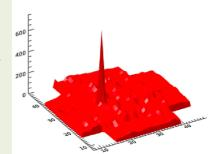
Muon ring images: acquired by each single Cherenkov camera during normal data taking, allow us to evaluate the optical throughput and to monitor the PSF.
