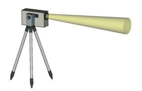
*lluminator:* a portable ground-based device designed to uniformly illuminate the telescope's aperture with a pulsed or continuous reference photon flux. It will be used, whenever necessary, to perform the absolute end-to-end calibration of each telescope of the ASTRI-MA.
