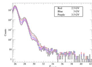
**Figure 3(a):** Variation in Z due to different minimum cutoff rigidity, bin size in 0.1 units of charge. Minimum cutoff rigidity ranges from 2-4 GV with 2.5 in red, 3 GV in blue, and 3.5 GV in purple.
