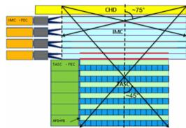
**Figure 1(b):** CALET side-view showing CHD, IMC, and TASC detector placement with the maximum acceptance angles for detection. In the UH trigger analysis this is  $75^\circ$  and in the TASC analysis this is  $45^\circ$ .
