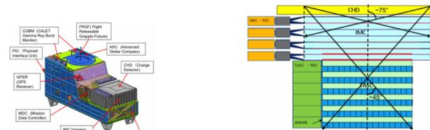
**Figure 1(a):** CALET instrument package detailing location of various CALET subsystems.
