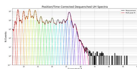
**Figure 3(b):** Charge histogram produced through L-Shell determination of rigidity. Minimum rigidity threshold of 4 GV bin size in 0.1 units of charge.
