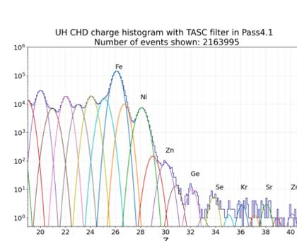
**Figure 5(a):** UHCR TASC analysis histogram with multiple gaussian fitting, bin size in 0.1 units of charge.
