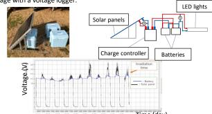
Result: When the output voltage from the solar panel increased, the output voltage of the battery also increased. Therefore, the power supply system was found to be working properly. It was also found that the output voltage of the battery was about  $12V \pm 2V$ .
