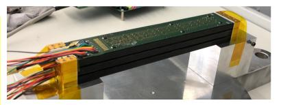
The **MAPS technology** for the HEDP-02 tracker has been **fully qualified for space applications**, successfully passing radiation hardness tests, electrical tests, mechanical and thermal stress tests (picture: turret ready for vibration tests)
