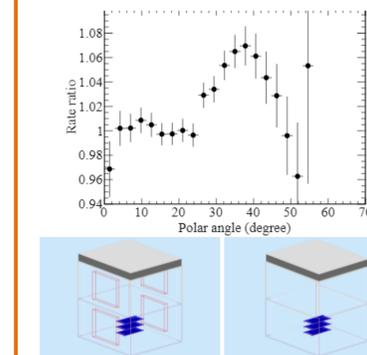
In addition to the effects due to the material overlying the telescopes, lateral obstacles such as the presence of a wall or the presence of a window near the detector must also be considered. Simulation results show that even such a little detail affects the measured angular distributions. Such a significant sensitivity, is an interesting feature that demonstrates how muons can be used to perform a scan of surrounding materials (muon tomography [12]).
