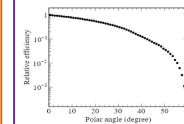
The relative detection efficiency, obtained as the ratio of detected and generated muons, as a function of the polar angle (left) for outdoor telescope, and muons generated in the full energy range (0.2-100 GeV). The distribution has been normalized to the value corresponding to vertical tracks.
