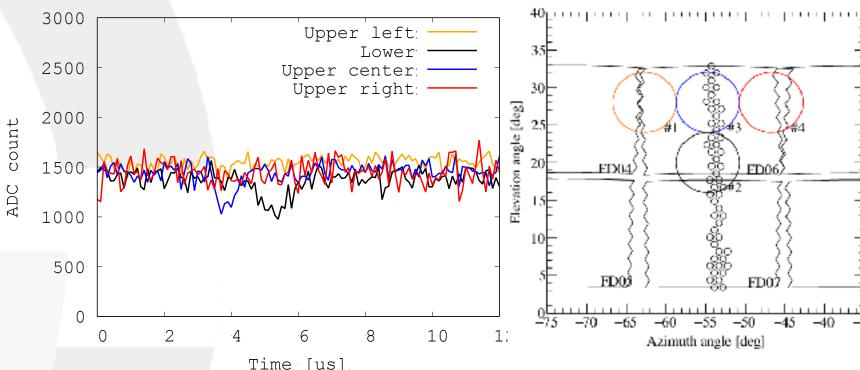
Fig2. Air shower event detected by CRAFFT at TA site. (E=10<sup>17.7</sup> eV, 3.6 km apart from the detector analyzed by TA FD)
