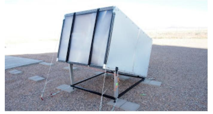
Fig1. Exterior of CRAFFT detector which consists of Fresnel lens, UV trans. Filter, 8 inc. PMT, FADC.
