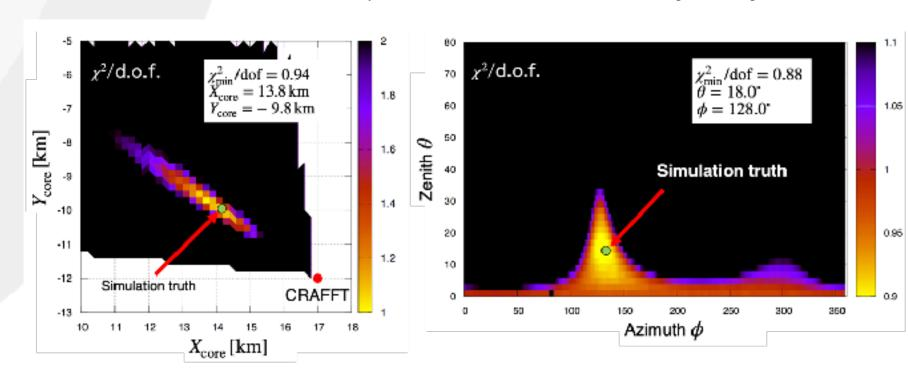
Fig3. Reduced chi<sup>2</sup> distribution for geometry reconstruction by waveform fitting. (Simulation study) chi<sup>2</sup> is converged around true value.
