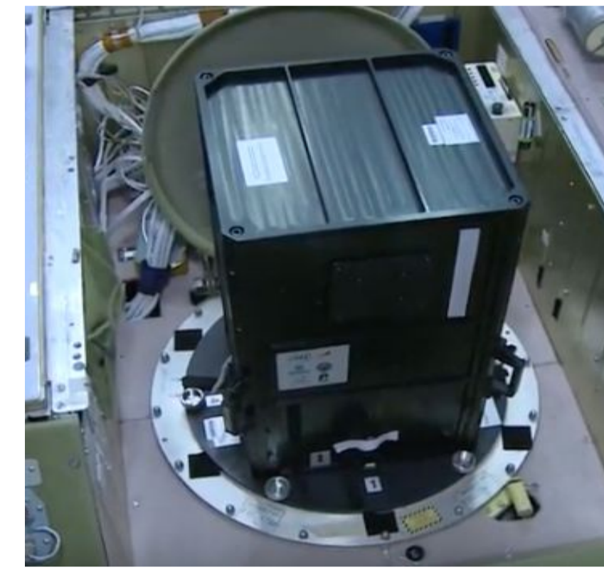
Mini-EUSO during a data acquisition session onboard the International Space Station, installed on the UV transparent window of the Zvezda module [1]
