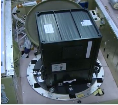
Mini-EUSO during a data acquisition session onboard the International Space Station, installed on the UV transparent window of the Zvezda module
