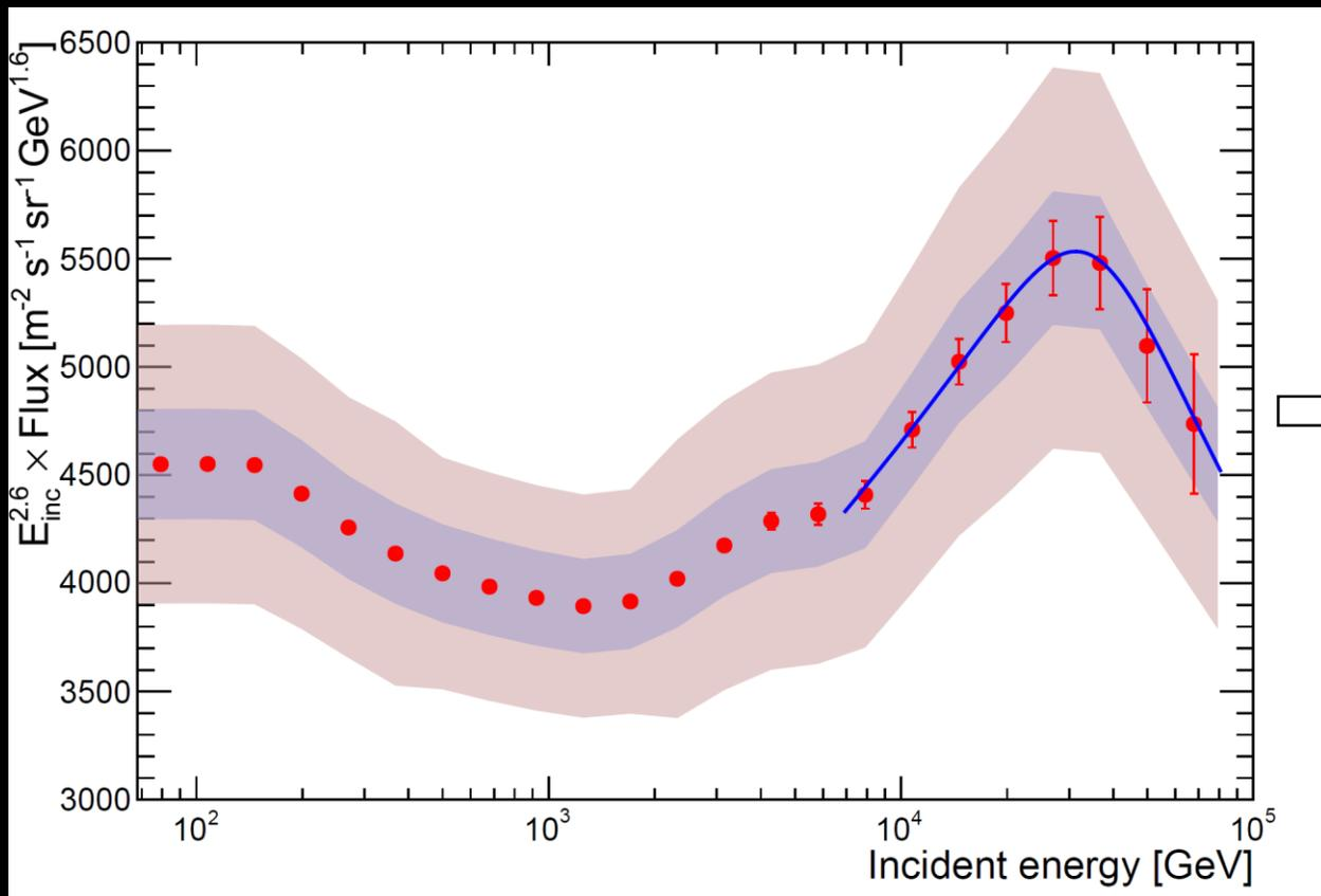
Fit of the softening structure with a Smoothly Broken Power-Law (SBPL) in the energy range [6.8 TeV - 80 TeV].
