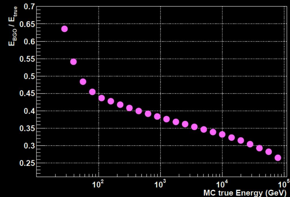
The limited thickness of the DAMPE calorimeter ( $\sim 1.62$  nuclear interaction lengths) significantly affects the energy response. In fact, only a part of the total particle energy is deposited inside the detector ( $\sim 40\%$  at 10 TeV), decreasing with the true energy due to a deeper development of the showers inside the calorimeter.
