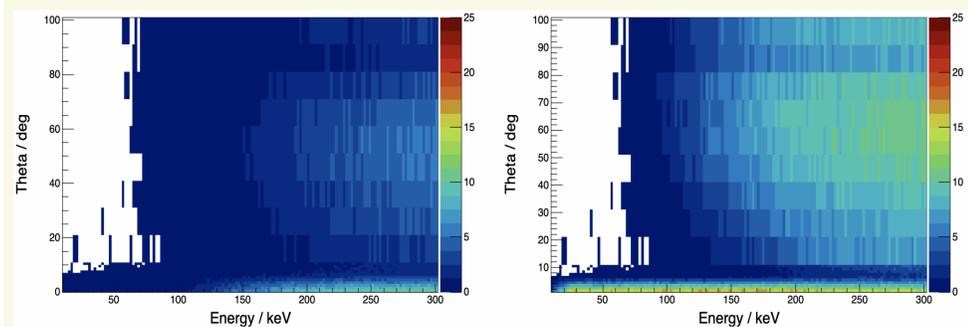
**Figure 3:** Effective area as a function of theta and energy (one tube). The left plot is for obscured tube, and the right is for opened tube.
