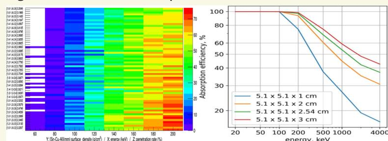
**Figure 2:** Left: transparency of collimator with different thicknesses. Right: absorption efficiency v.s. energy for different thicknesses of CeBr<sub>3</sub> [9].
