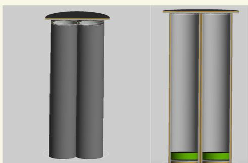
**Figure 1:** A simplified construction drawn by [8]. Left: the shutter and four collimated spectrometers. Right: a vertical section of them, where you can see the layers of collimators, and inside spectrometer modules. One tube: diameter 51 mm, length 500 mm, FoV 26 deg<sup>2</sup>.
