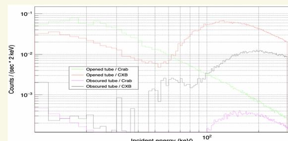
**Figure 4:** Predicted count rate spectrum of both the CXB and the Crab pulsar (one tube). Different colors are represented for different tubes & sources.
