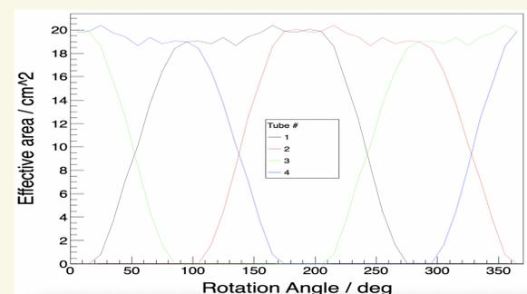
**Figure 5:** The changing of effective area with the rotation phase of obturator.
