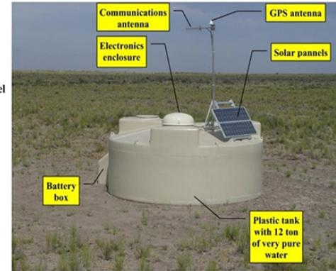
The Cherenkov signals in each SD station are collected by three PMTs and digitised using 40 MHz, 10-bit Flash Analog-to-Digital Converters (FADCs).
