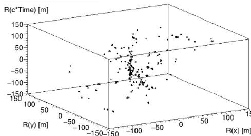
Figure 3.8: EAS in rotated Coordinate point cloud, the hough line found for the rotation illustrate no concise vertical.
