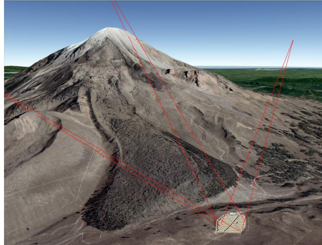
*Muon trajectories with differing offsets for three arrival directions.*
