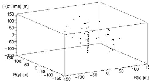
Figure 3.7: Single Muon in rotated coordinate point cloud, points associated with the muon are localized to the vertical line.
