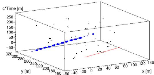
Figure 3.5: Event point cloud with a single muon (blue points)
