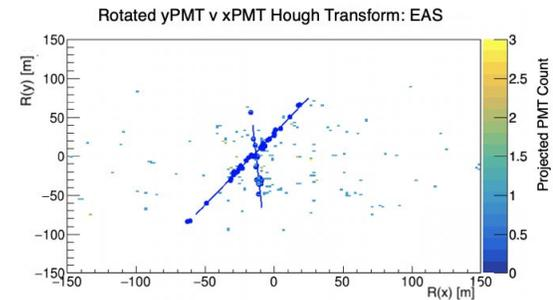
Figure 3.10: Projected 3D Hough Transform for EAS plane, an initial line is found in the plane and when rotated to it it then allows for the plane to be found in a second line.
