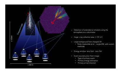
Figure: Imaging atmospheric Cherenkov telescope technique.
